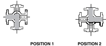
FLOW PLAN N - 4-WAY L PORT 180° TURN
